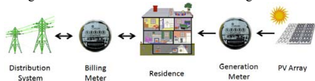
Fig. 7. Net metering scheme for proposed scheme
